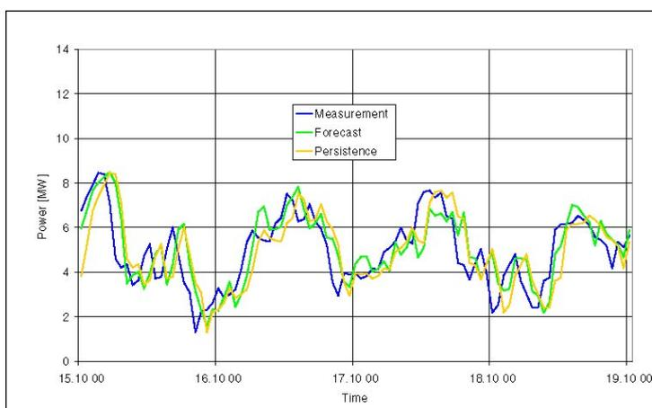
Figure: Measured and predicted power output of wind farm Bears down
