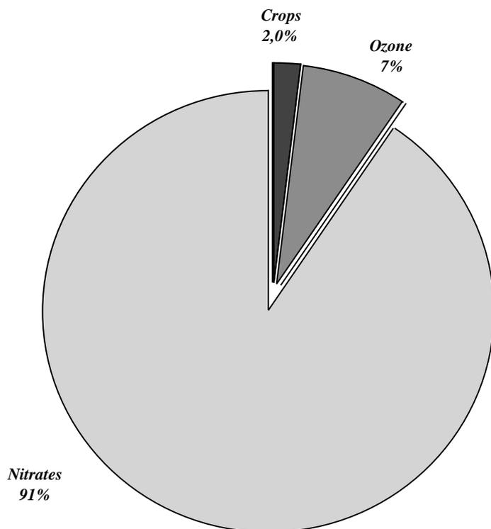
**Figure 4.5:** Breakdown of damage costs, excluding global warming, by pollutant for the natural gas power plant in Cordemais near Nantes, France. Total = 11.4 mECU/kWh<sub>el</sub>.
