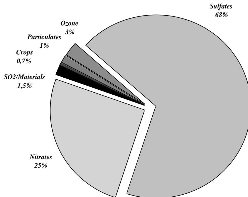
**Figure 4.7:** Breakdown of damage costs, excluding global warming, by pollutant for the oil fuel power plant in Cordemais near Nantes, France. Total = 68.7 mECU/kWh<sub>el</sub>.
