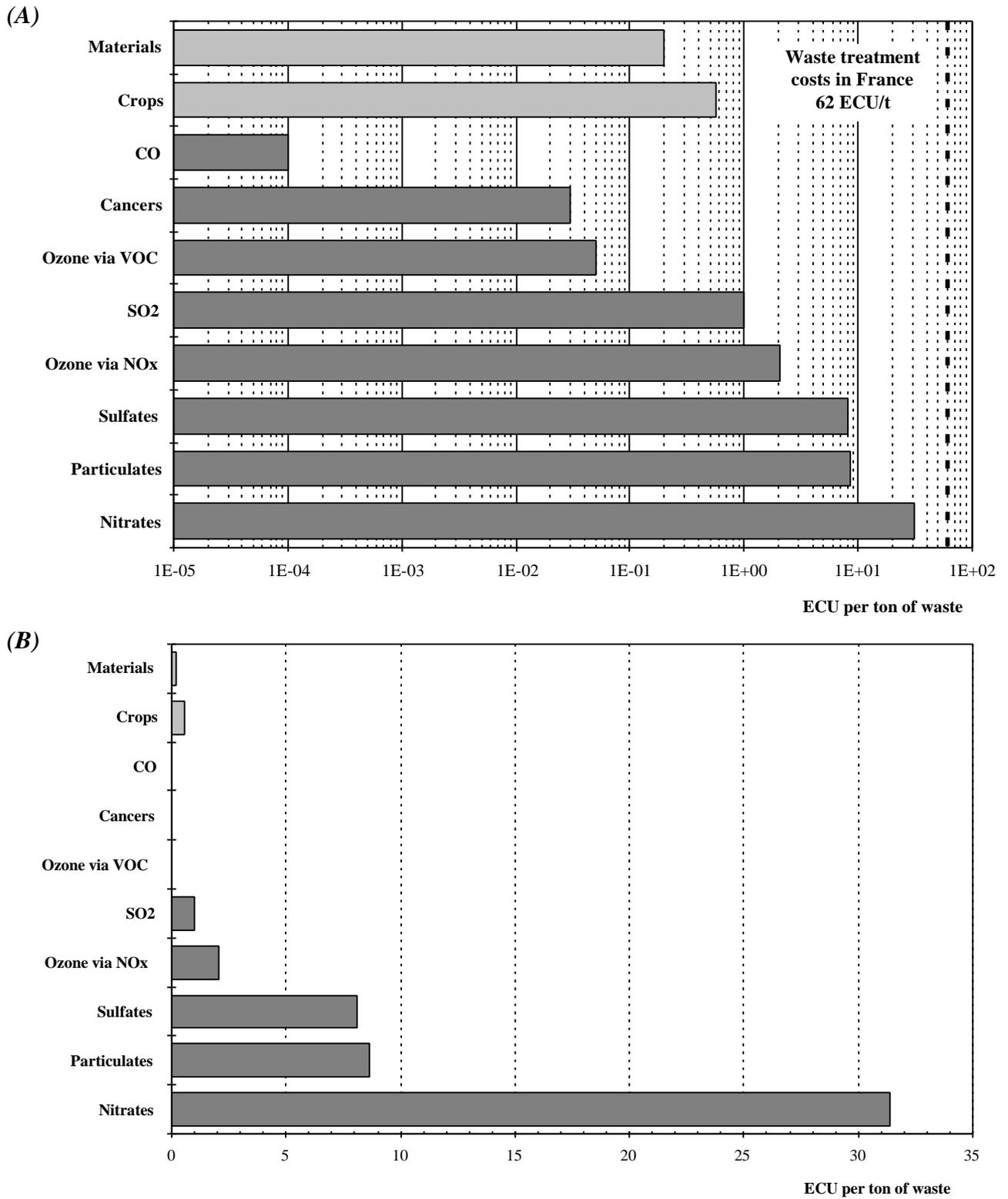
Figure 4.15: Damage costs (incineration stage only) for the MSW incinerator in Paris, France.
