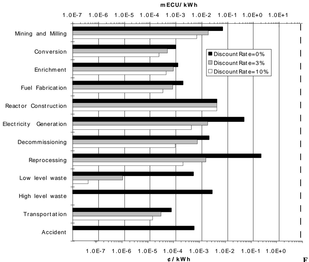
**ig.ES.4.** Damage cost for the **nuclear** fuel cycle, by stage of cycle, for three discount rates: 0% (black), 3% (gray), and 10% (white).
