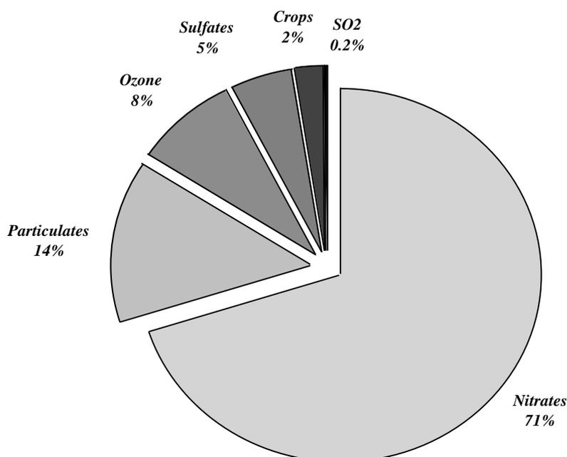
**Figure 4.9:** Breakdown of damage costs, excluding global warming, by pollutant for the biomass plant in Albi near Toulouse, France (upstream/downstream and power production stages included). Total = 5.5 mECU/kWh<sub>el</sub>.
