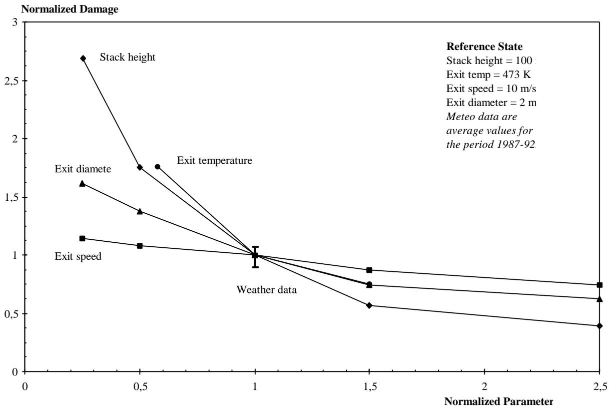
**Figure 5.1:** Influence of emission source parameters and meteorological data on damage estimates. The source is located in a suburb of Paris.
