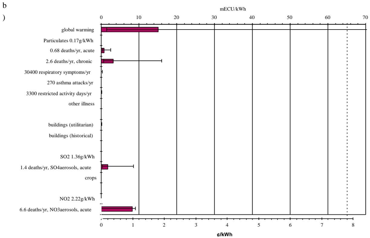
**Fig.ES.2.** Quantified impacts/year and costs (with uncertainties) for **coal** fuel cycle: intermediate load power plant at Cordemais, output  $2.1 \times 10^9$  kWh/yr. Dashed line = average retail price 65 mECU/kWh. a) logarithmic scale b) linear scale
