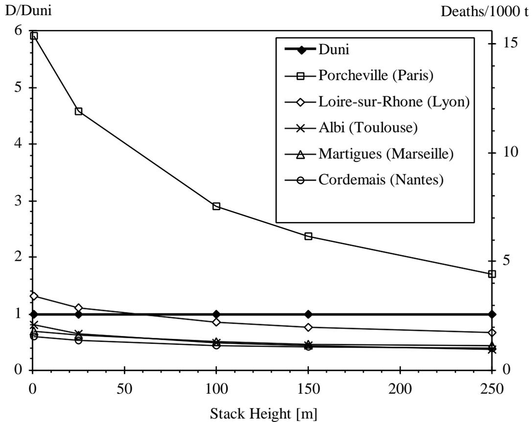
**Fig.ES3.** An example of dependence on site and on height of source for a primary pollutant: damage  $D$  from  $SO_2$  emissions with **linear dose-response function**, for five sites in France, in units of  $D_{uni}$  for uniform world model Eq.1 (the nearest big city, 25 to 50 km away, is indicated in parentheses). The scale on the right indicates deaths/yr (acute mortality) from a plant with emission 1000 ton/yr.
