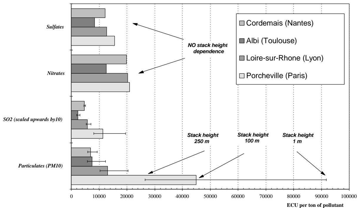
**Figure 5.2:** Damage costs per ton of pollutant for different sites across France. The reference emission stack height is 100 m. Impacts include costs for health, crops and building surfaces.
