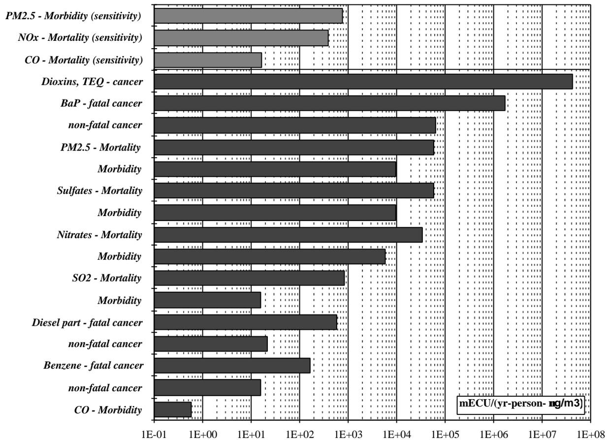
**Figure 3.1:** Comparison of air pollution health impacts in terms of cost per ambient concentration of the respective pollutant. The items labeled “*sensitivity*” correspond to ER functions that are considered less well established and that have not been used in the present work.
