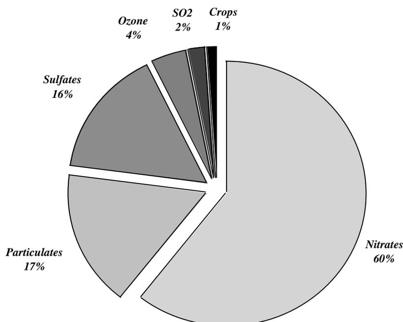
**Figure 4.14:** Breakdown of damage costs by pollutant for the MSW incinerator in Paris (excluding global warming). Total = 51.9 ECU per ton of waste.
