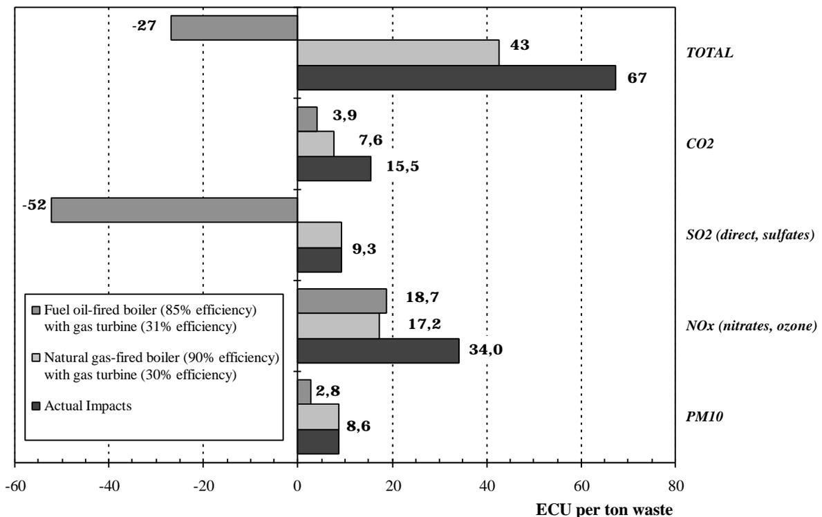
**Figure 4.16:** Avoided emissions and damage costs for recovered heat and electricity production using two different displaced technologies (Paris MSW incinerator). Global warming impacts are valued at 18 ECU per ton CO<sub>2</sub>.
