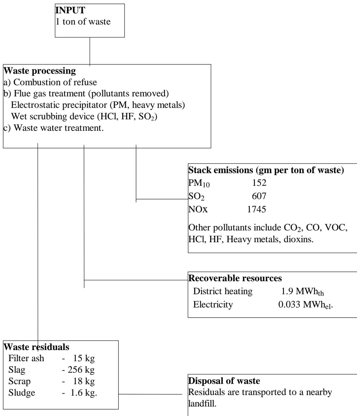
Figure 4.13: Stages for waste incineration.
