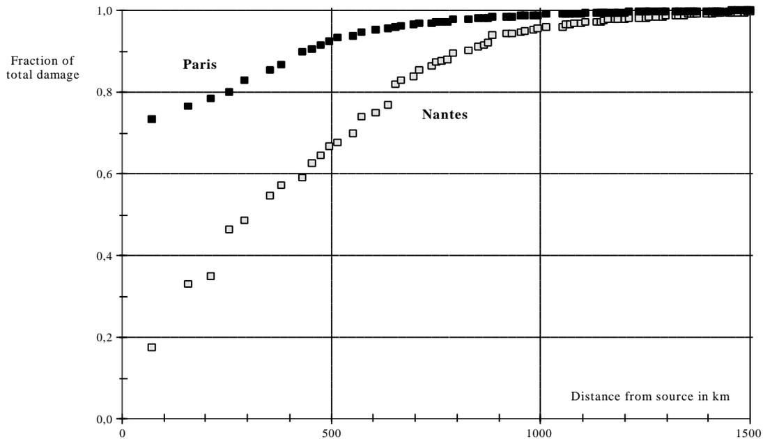
**Figure 5.4:** Variation of “primary” particulate damage with distance from source and geographic impact range for two French sites (reference stack height is 100 m).
