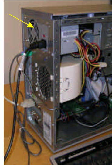
View of a power supply in a desktop PC
