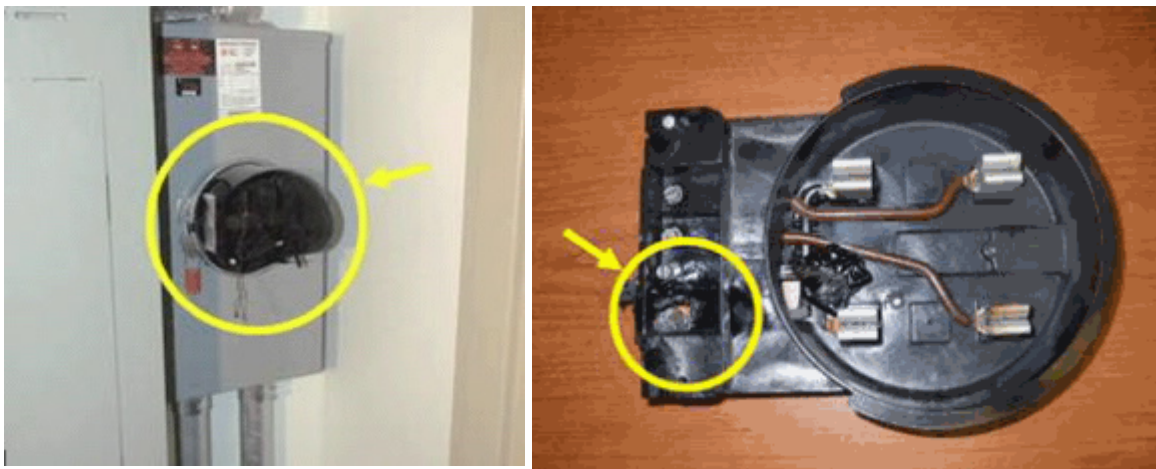
Meter explosion; base plate remained intact
