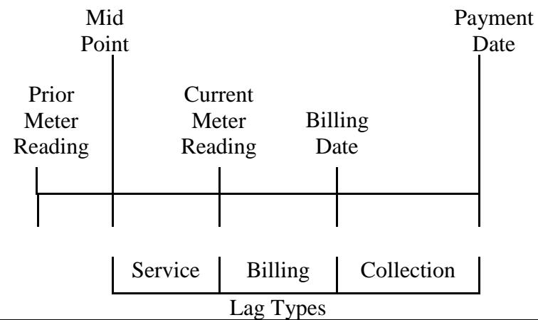
Meter reading: On this date two important events occur. The past service period ends and the new service period begins. The differences between the prior read and the current read measures the volumes delivered over that time period.
