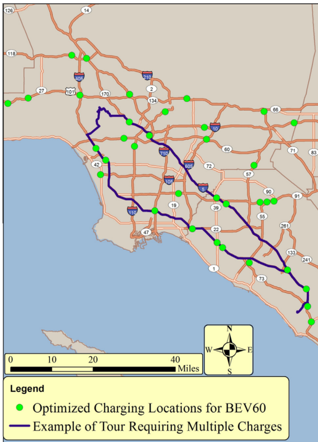
Fig. 8. An example tour for a vehicle requiring multiple fast charging events.
