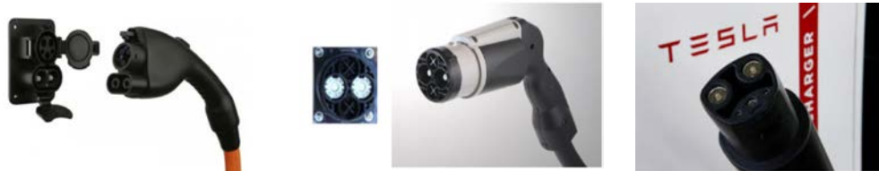
Figure 5. DC fast charging connector standards and compatibility
